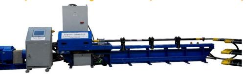
The Dyno-Master provides after redress, pre-run and post run motor performance verification.
